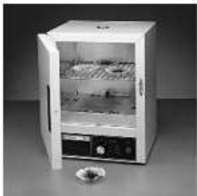
Conventional laboratory oven used for drying materials.
