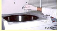
Centrifuge the mixture for 5 minutes at 500 g (~2000rpm).
