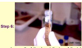
Loosen the fatty plug at the top of the tube with an applicator stick and invert the tube to discard the supernatant.
