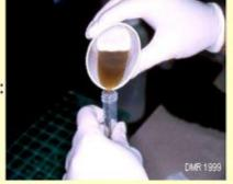
Pour the filtrate into a 15 ml centrifuge tube and add 3 ml of ethyl acetate, mix well (~1 min) by hand.
